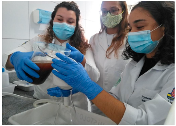
Figure 12: Sample vacuum filtration process after chemical digestion process of S. guianensis food content (Photo: Aquasis).
